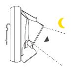
The intensity and the direction of the light beam are managed automatically by means of an environment light sensor: it avoids optical harm among the users and saves battery duration.
